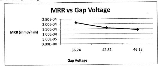
Figure 9: Material Removal Rate versus Gap Voltage
