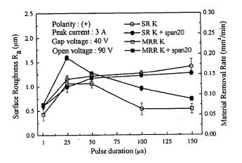
Figure 3: Influence of pulse duration on surface roughness and material removal rate: (SR) Surface roughness, (MRR) Material Removal Rate, and (K) kerosene
