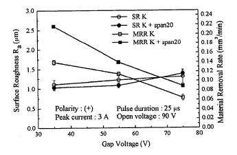
Figure 2: Influence of gap voltage on surface roughness and material removal rate: (SR) Surface roughness, (MRR) Material Removal Rate, and (K) kerosene
