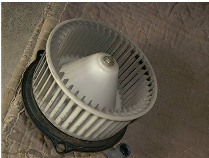
Figure 2.2: Squirrel cage fan that used to help move air throughout the passenger compartment.
