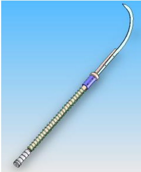
Figure 3 : Subassembly of the Sickle & Sliding Shaft
