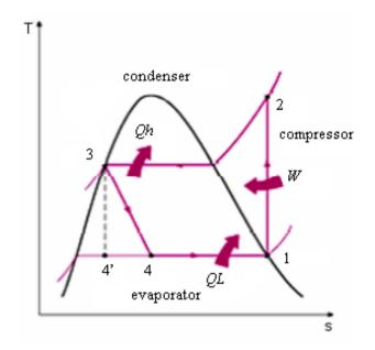
Figure 2.1: T-s diagram for the ideal vapor compression cycle [8]
