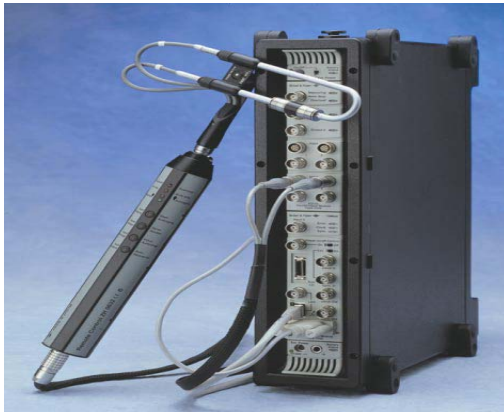
Figure 3: Digital signal analyzer, probe and microphone
