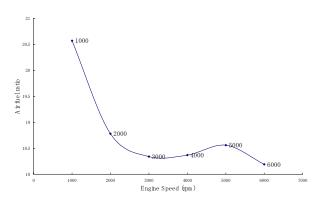
Figure 7: Air fuel ratio at different engine speed
