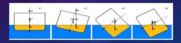
Liquefaction which reduces ship's positive stability and metacentric height (GM) may cause possible loss of the ship [8].
