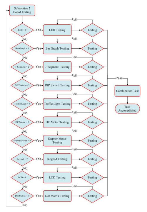
Figure 4: Application Module Testing Flow
