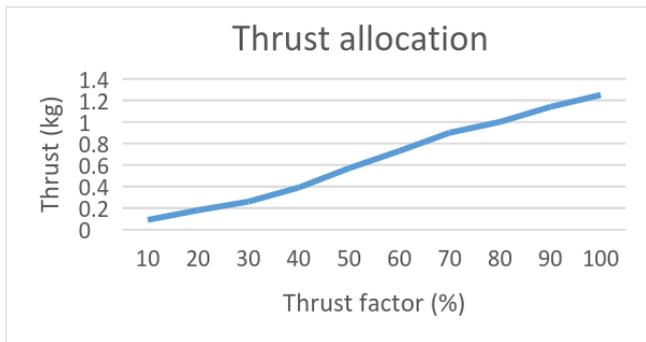
Fig. 13. Thrust in the water
