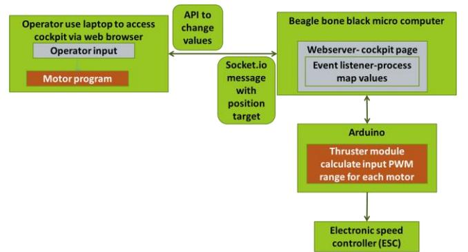
Fig. 8. The ROV system architecture
