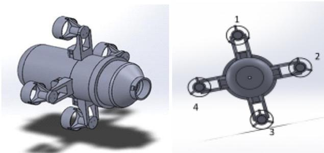
Fig. 3. SolidWorks drawing for X4-ROV
