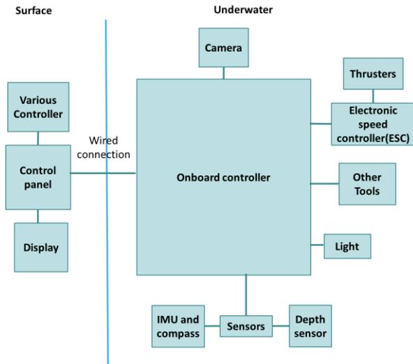
Fig. 7. Electronic system block diagram
