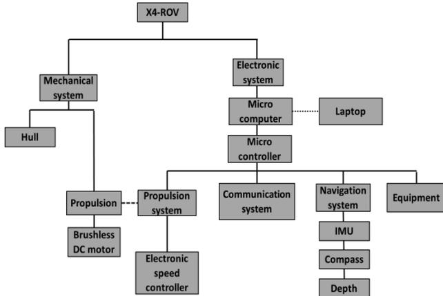
Fig. 1. X4-ROV system
