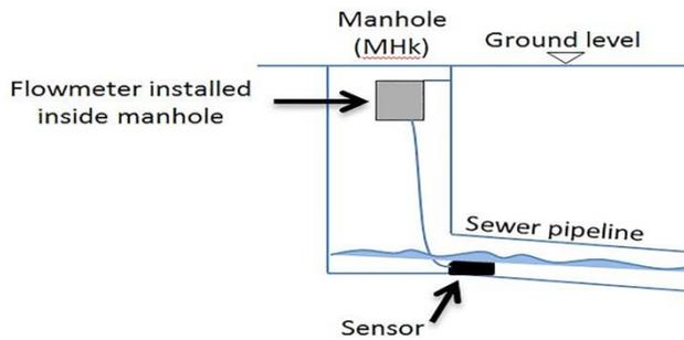
**Figure 2.** Sensor attached with flow meter and installed in selected manhole.
