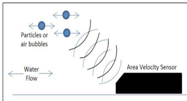
Figure 1. Ultrasonic technology sensor.
