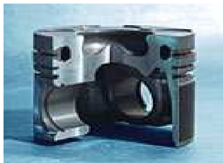
Figure 2.10: Pistons with cooled ring carriers.
