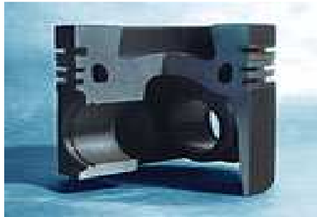
Figure 2.9: Ring carrier pistons with cooling channel and crown reinforcement
