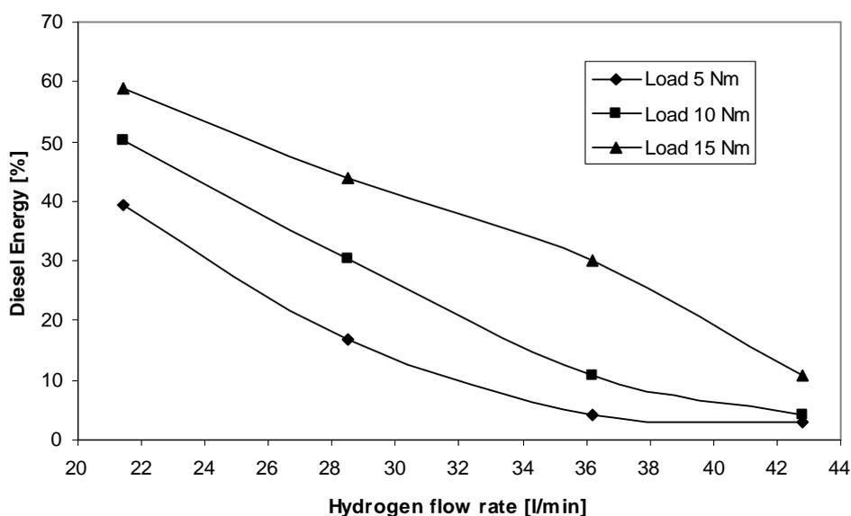
Figure 2: Diesel energy replacement by hydrogen
