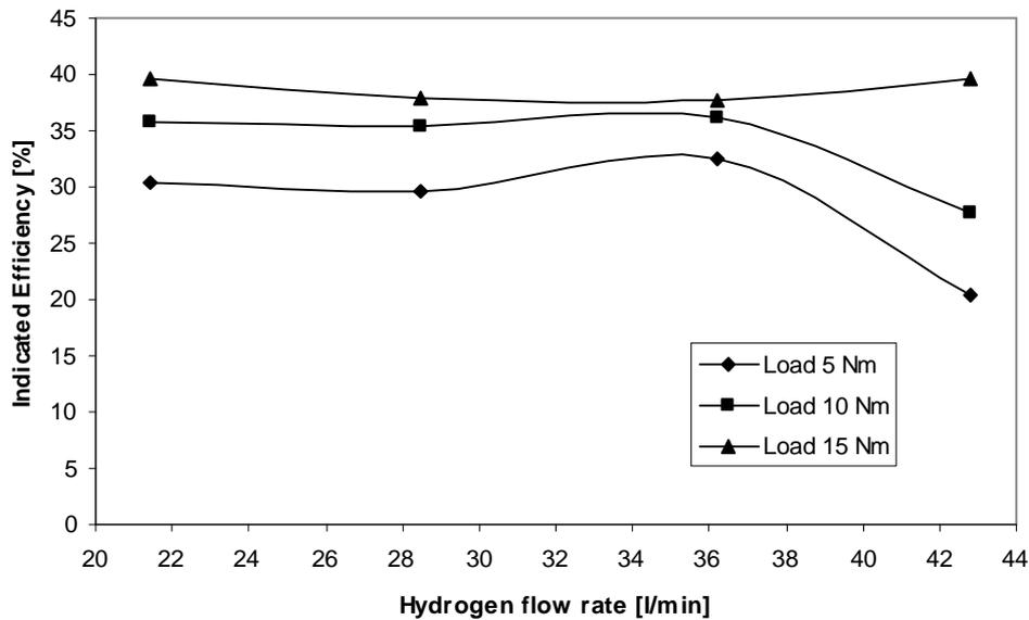
Figure 5: Variation of indicated efficiency with hydrogen enrichment and load
