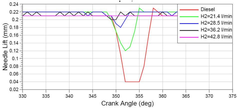
Figure 3: Needle lift at 2000 rpm, 5 Nm
