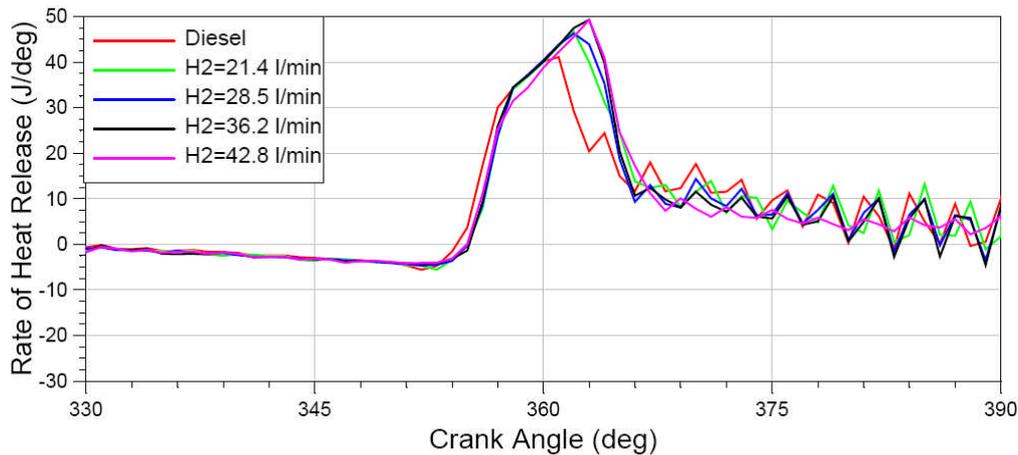
Figure 11: Rate of heat release at 2000 rpm, 15 Nm
