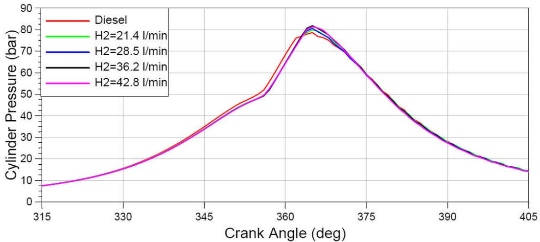
Figure 10: Cylinder pressure at 2000 rpm, 15 Nm
