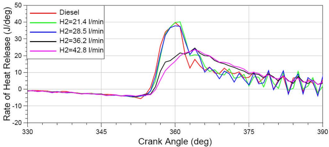
Figure 9: Rate of heat release at 2000 rpm, 10 Nm
