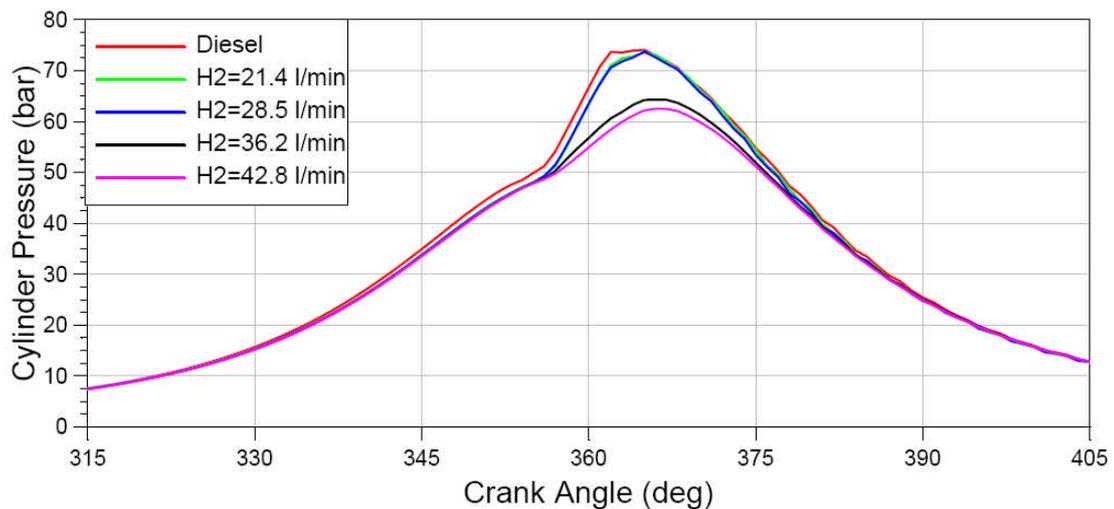
Figure 8: Cylinder pressure at 2000 rpm, 10 Nm
