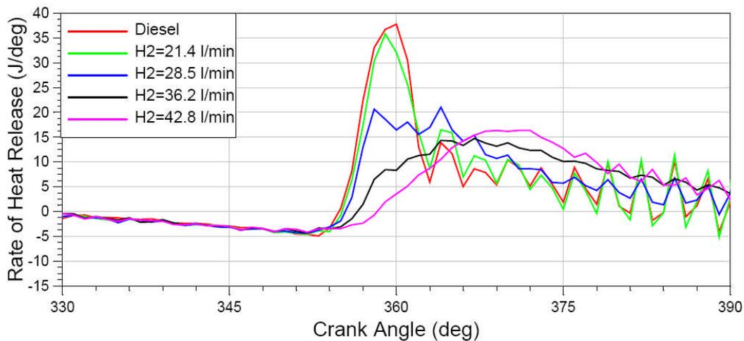
Figure 7: Rate of heat release at 2000 rpm, 5 Nm
