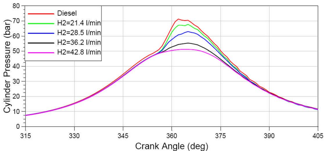
Figure 6: Cylinder pressure at 2000 rpm and 5 Nm
