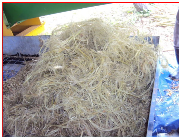
Figure 2: The greenish look kenaf fibre just from the Kenaf Decorticator Machine.
