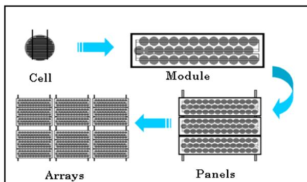
Figure 2.4: Transition of cell, module and arrays
