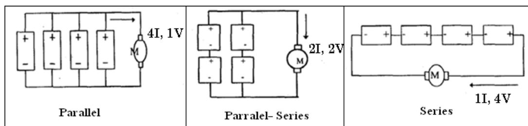
Figure 2.5: Three types of electrical array
