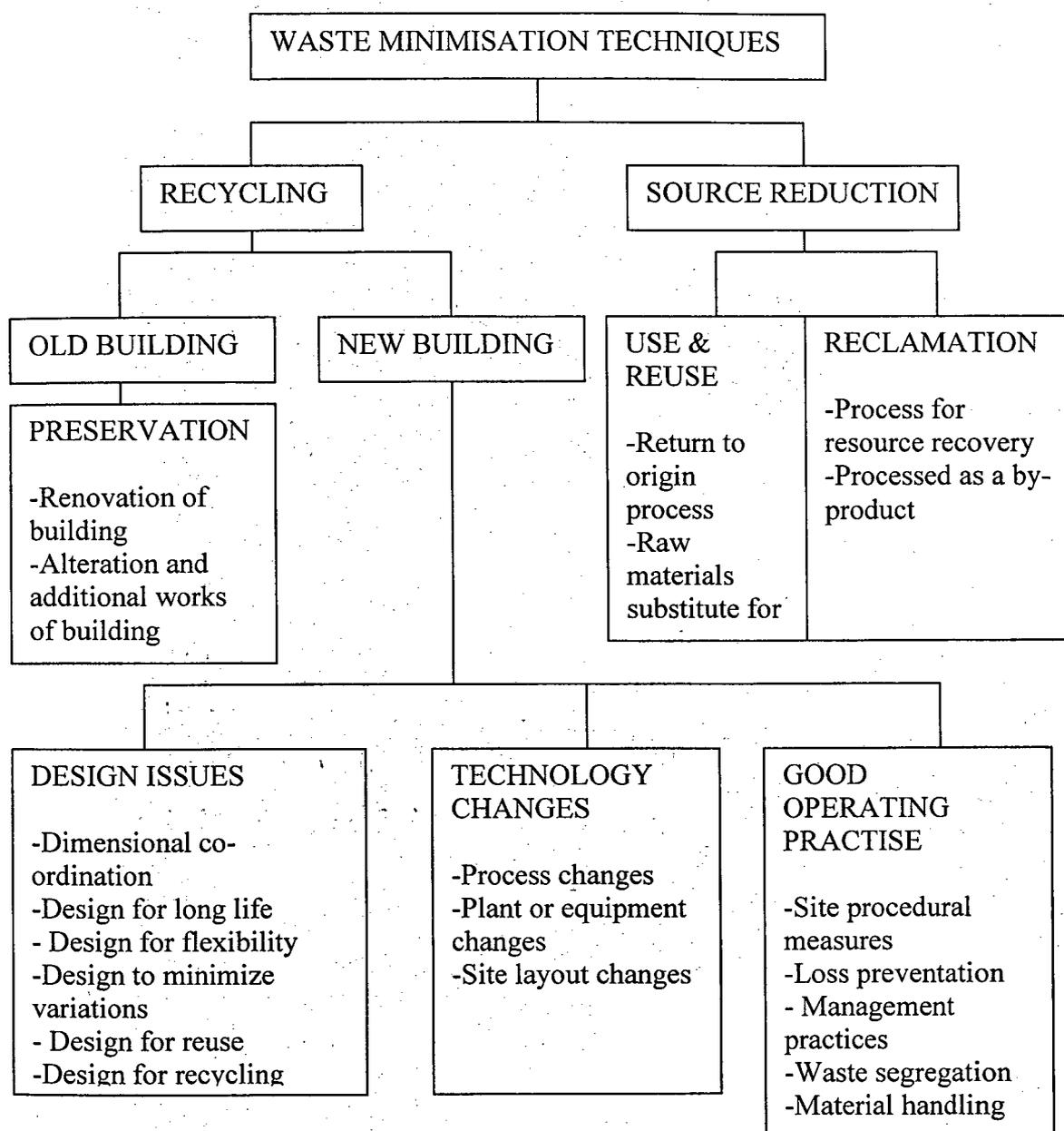
Figure 2.5: Waste Minimization Techniques in Construction (Modified from Ciambone, 1996)
