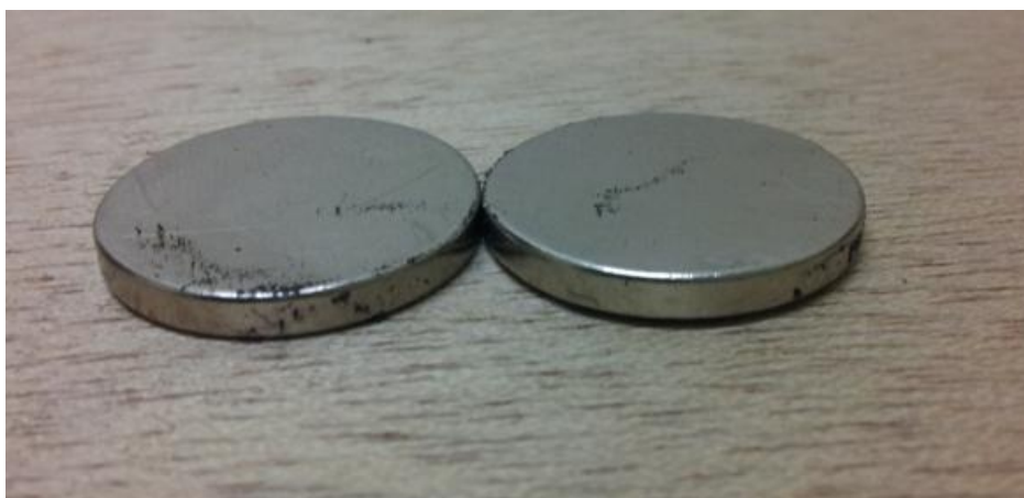
Figure 3.11: 1500-2000 Gauss Neodymium Magnet
