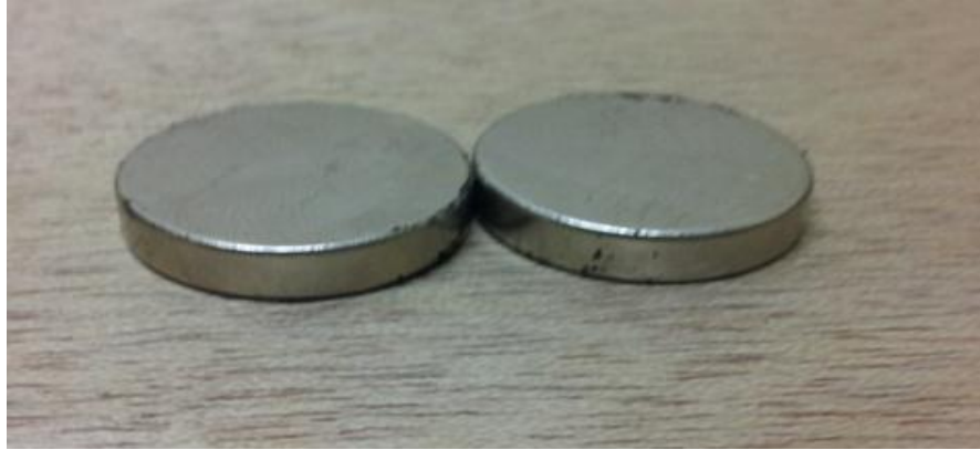
Figure 3.12: 2500-2800 Gauss Neodymium Magnet
