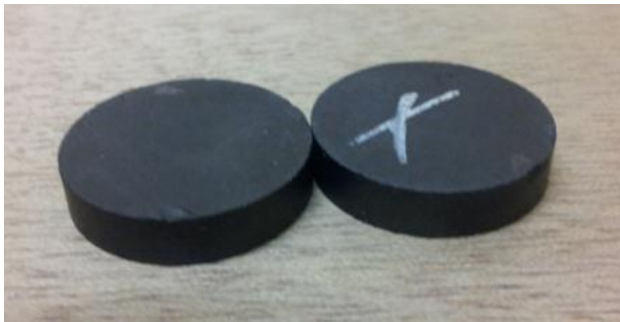
Figure 3.10: 500-800 Gauss Ferrite Magnet
