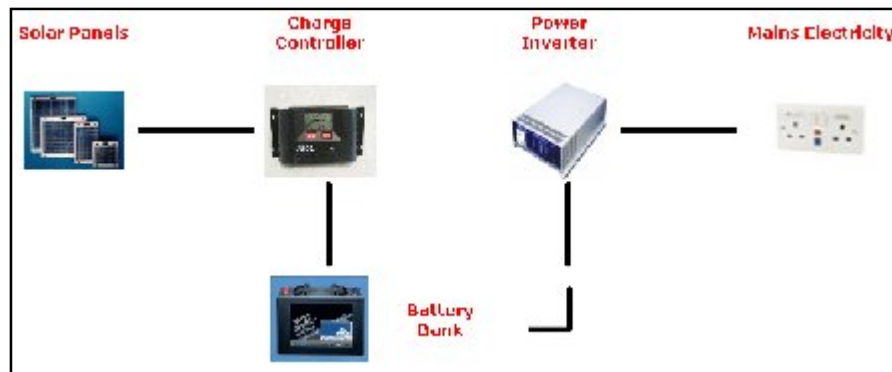
Figure 1.4 Block diagram for Photovoltaic Standalone System
