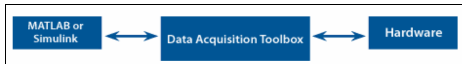
Figure 1: Connection between DAQ toolbox, hardware and MATLAB
