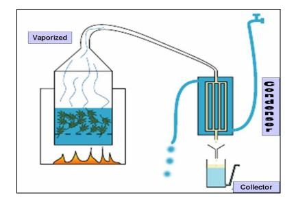
Figure 1.2: Simple Hydro Distillation Concept
