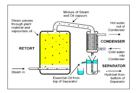
Figure 1.3: Simple Steam Distillation Unit
