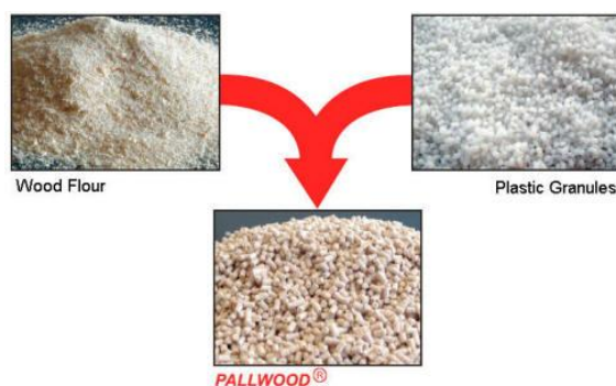
Figure 2.4: Combination of wood flour and plastic granule to form wood plastic composite.
