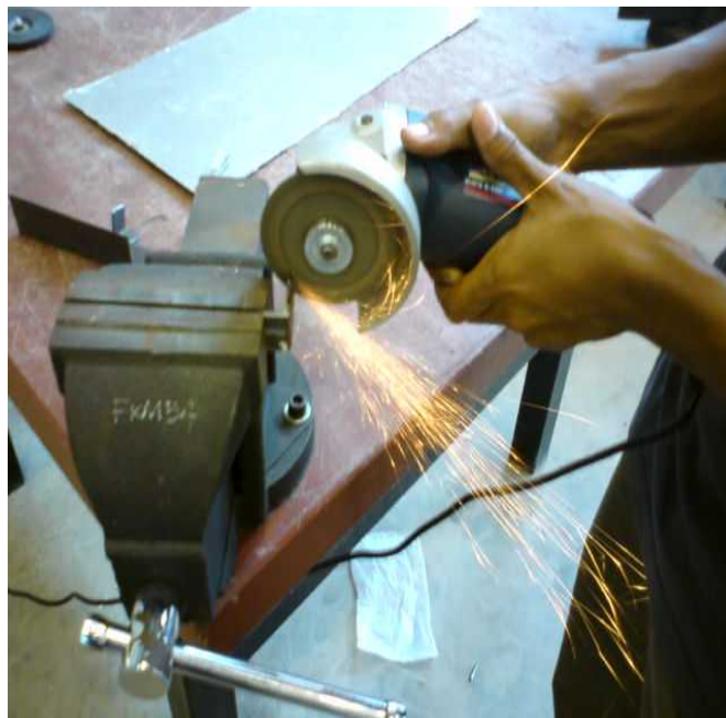
Figure 3.14: Finishing process using hand grinder
