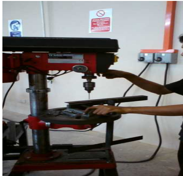
Figure 3.10: Using drilling machine to make a hole
