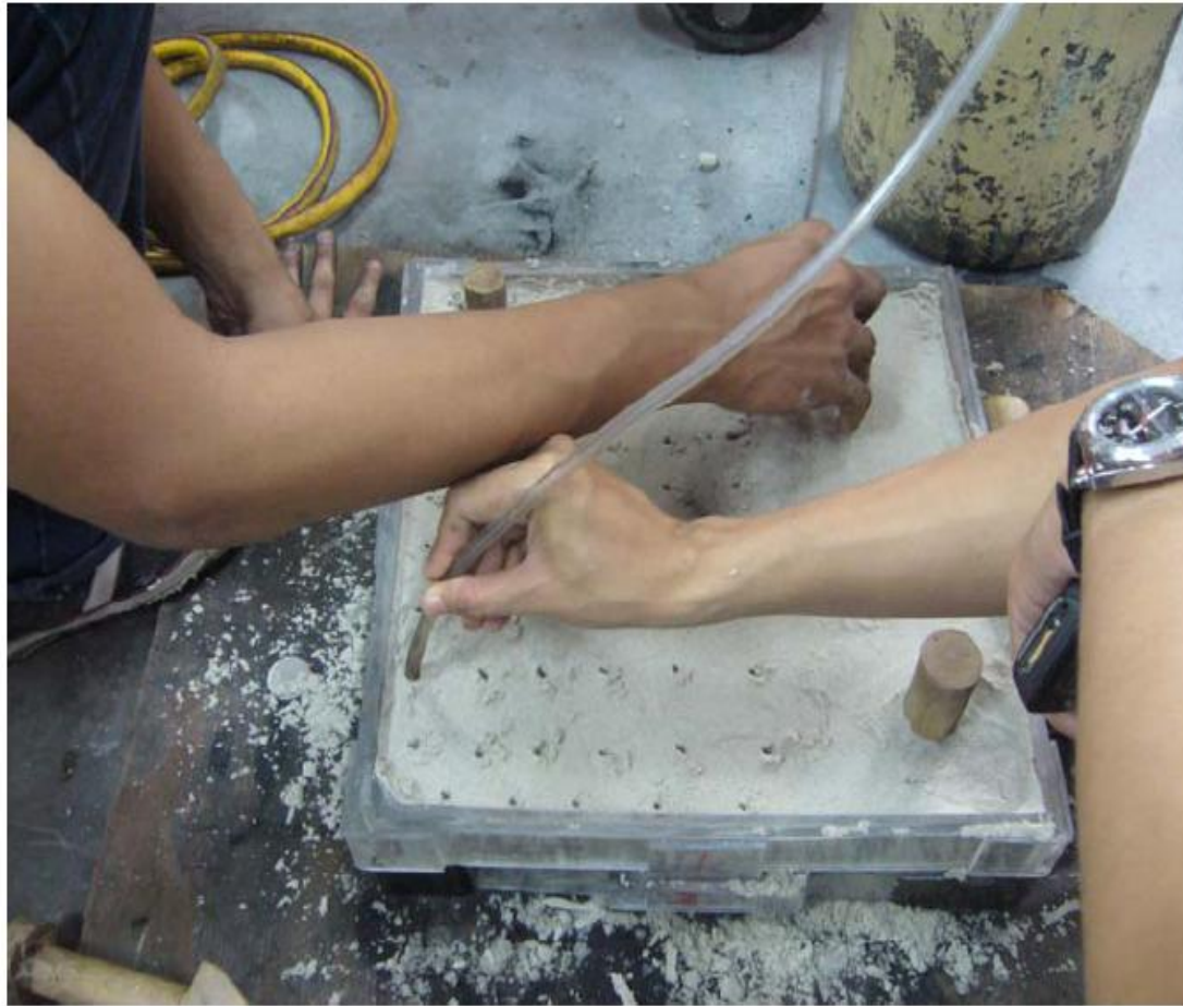
Figure 3.13: CO 2 Gas Being Spray into the Mold.
