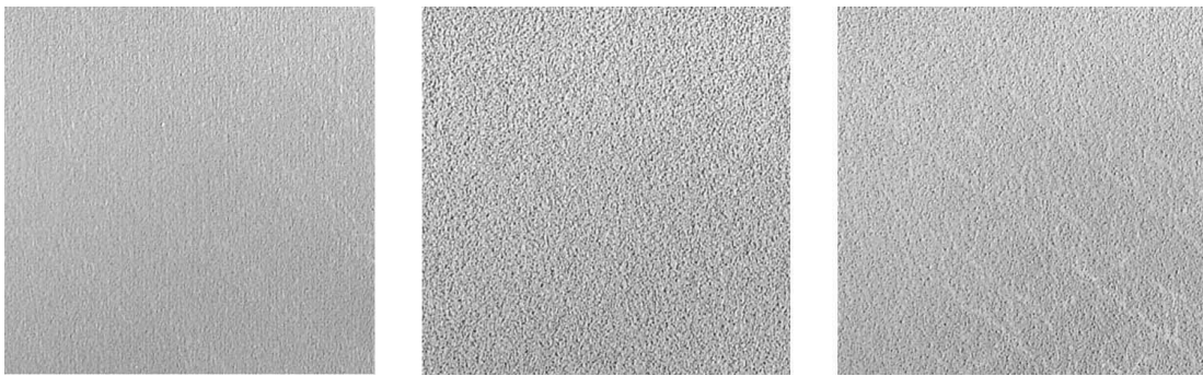
Figure 2.2: Surface roughness. These are photographs of pieces of sandpaper of varying grit painted the same shade of gray
