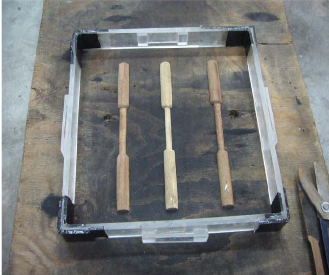
Figure 3.12: Split Dog Bone Pattern in the Molding Box.
