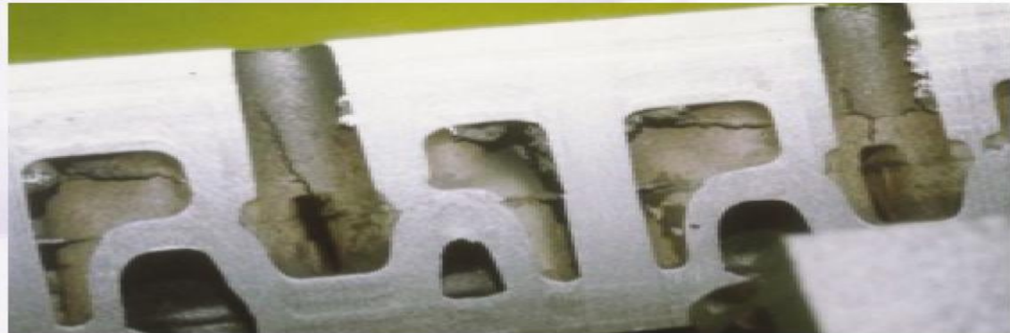
Figure 2.12: Example of Vein Defects in Cylinder Head
