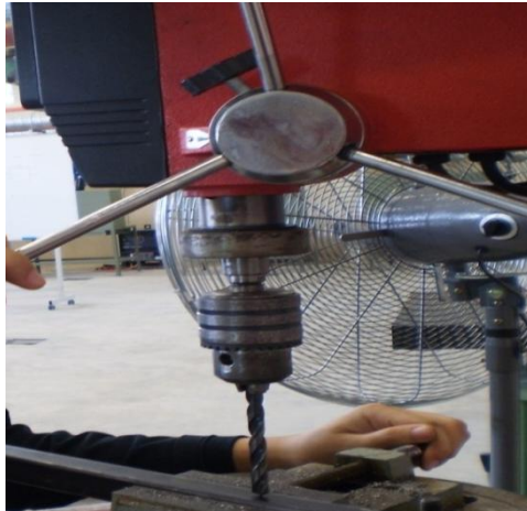
Figure 3.13: Process to make a hole
