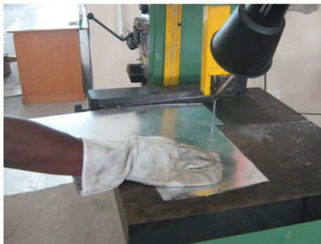
Figure 3.17: Cuts material using vertical bandsaw
