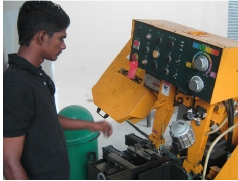
Figure 3.16: Cuts material using horizontal bend saw
