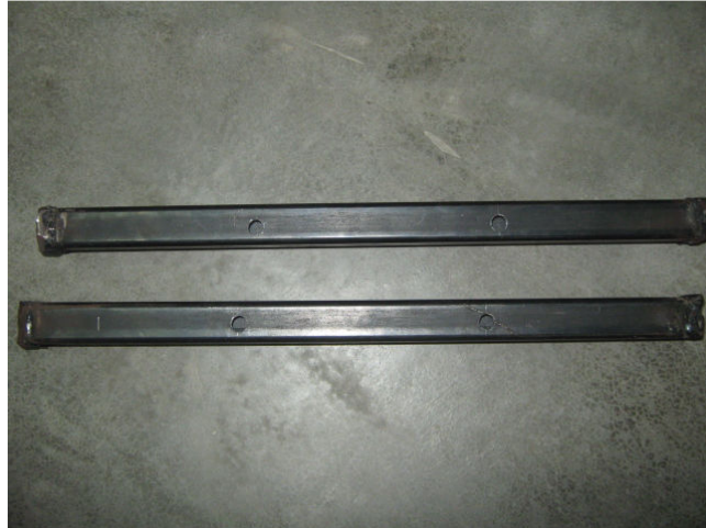
Figure 4.1 : Finished side clamping device
