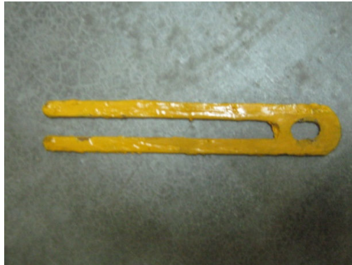
Figure 4.4 : Finished top clamping device
