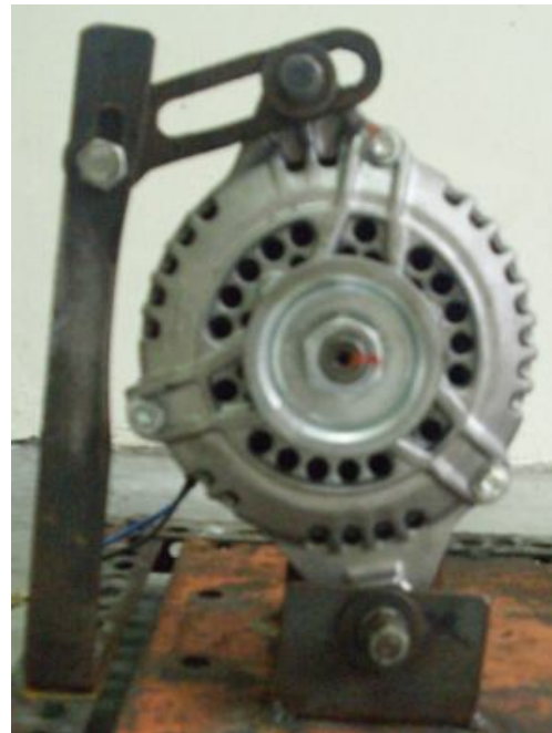
Fig 3.7: Installing the alternator
