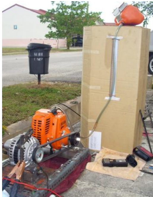
Fig 3.12: Engine test rig setup
