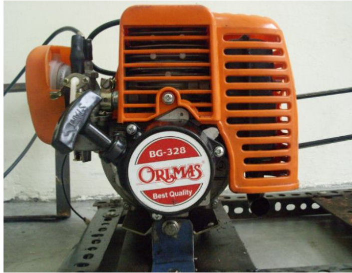
Fig 3.4: Small two stroke engine used
