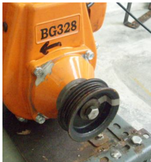
Fig 3.5: Modification on shaft by putting the pulley
