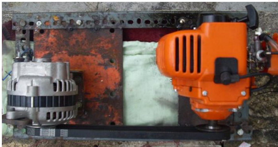
Fig 3.10: Upper view of engine test rig
