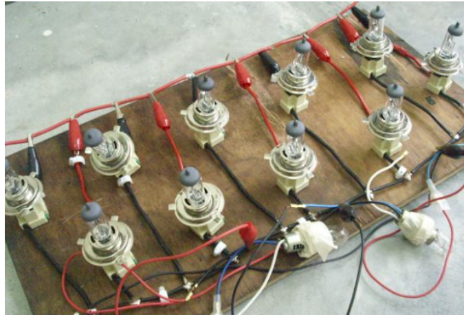
Fig 3.11: Electric circuit as load
