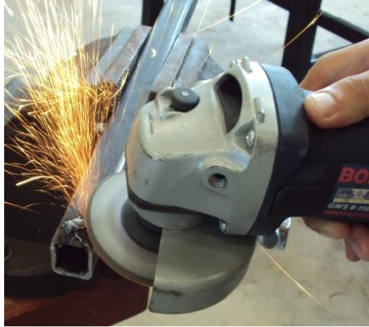
Figure 3.11: Grinding the joining point
