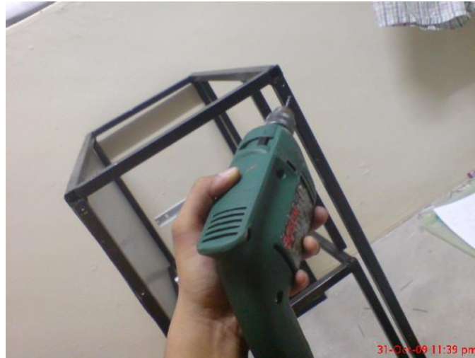
Figure 3.13: Drilling the rivet point
