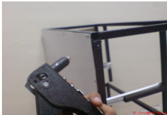
Figure 3.14: Rivet the zinc against body structure
