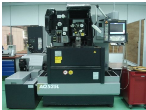
Figure 3.1: CNC Wire-cut Machine.
