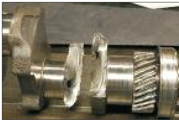
Figure 2.3: Fatigue failures on crankshaft
