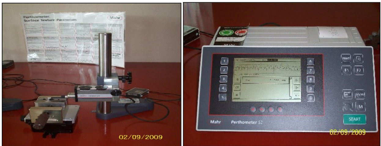
Figure 3.8: Perthometer S2 with surface roughness tester Mahrsurf XR 20
