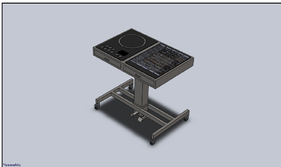
Figure 3.4: Cooking table with foot pump table lift.
