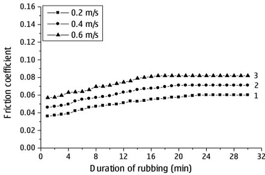
Fig. 7. Variation of friction coefficient with duration of rubbing at different sliding velocities (Normal load: 4 N, test sample: gear fiber, pin: SS 201)
