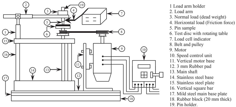
Fig. 1. Block diagram of the pin-on-disc experimental set-up
