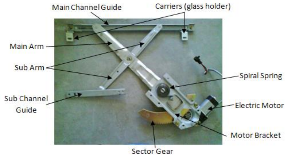
Figure 1.2: Integrated Scissor Type Regulator
