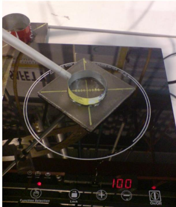
**Figure 3.14:** Steel Plate heated at 100°C
