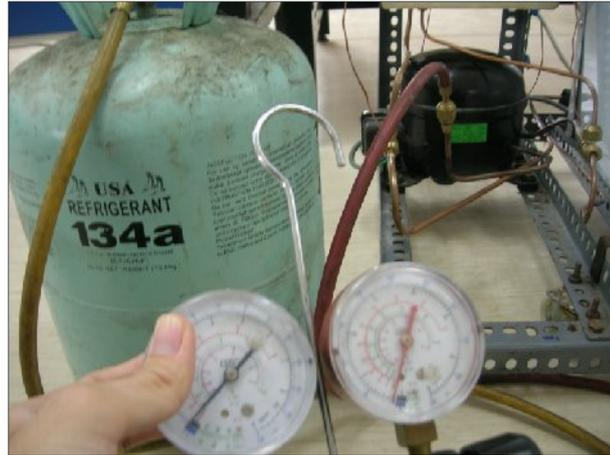
**Figure 3.11:** The refrigeration system test rig is being charged with refrigerant 134a
