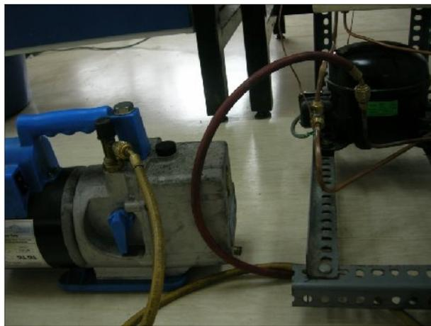
**Figure 3.10:** The refrigeration system test rig is being evacuated by vacuum pump
