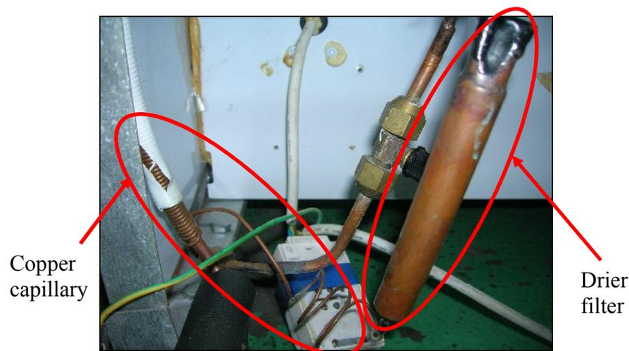
**Figure 2.7:** Copper capillary tube and drier filter
