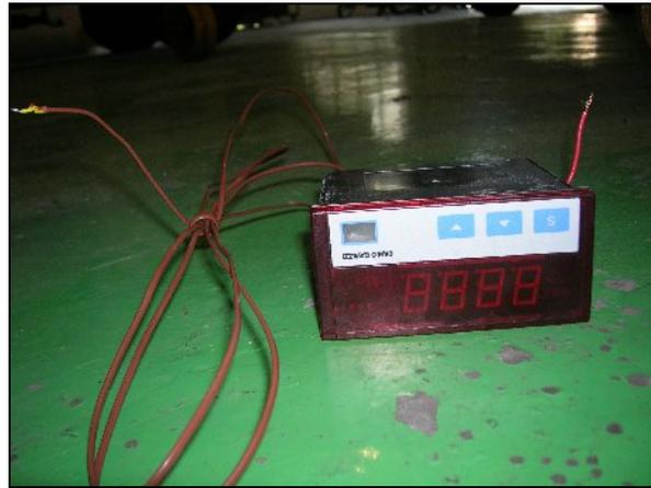
**Figure 2.11:** K type thermocouple that is used in this experiment
