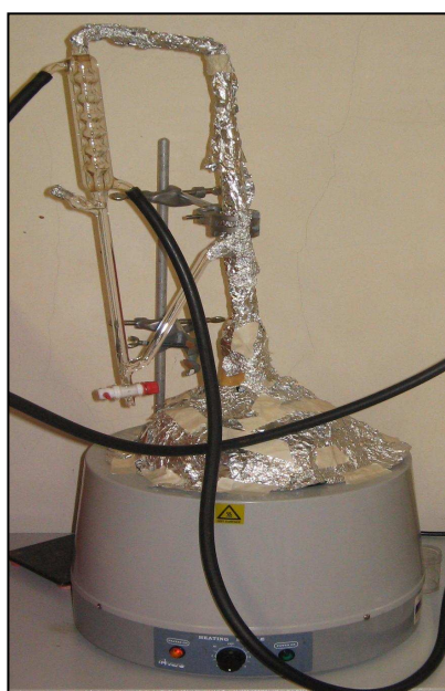
Figure 3.2 Clevenger-type hydro-distillation apparatus
