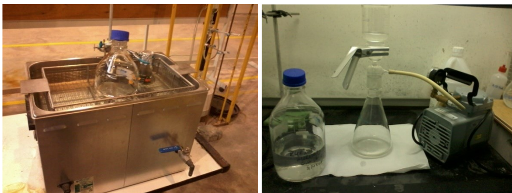
Figure A.2 Preparing the mobile phase (Degassed and filtered process)
