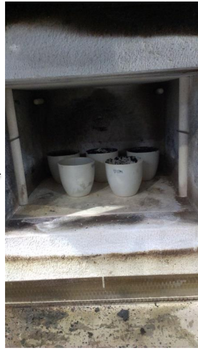
Carbonization with N 2 flow
