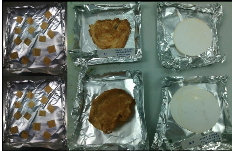
Figure 4-3: Observation on immobilized supports after 10 hours fermentation. (Process conditions: pH 5.0; 30 °C; 200 rpm; initial glucose concentration 150 gL -1 )
