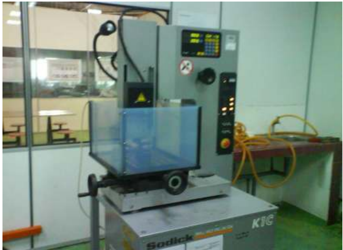
Figure 1: SODICK K1C EDM Micro Hole Drill Machine Installed at the Universiti Malaysia Pahang Laboratory
