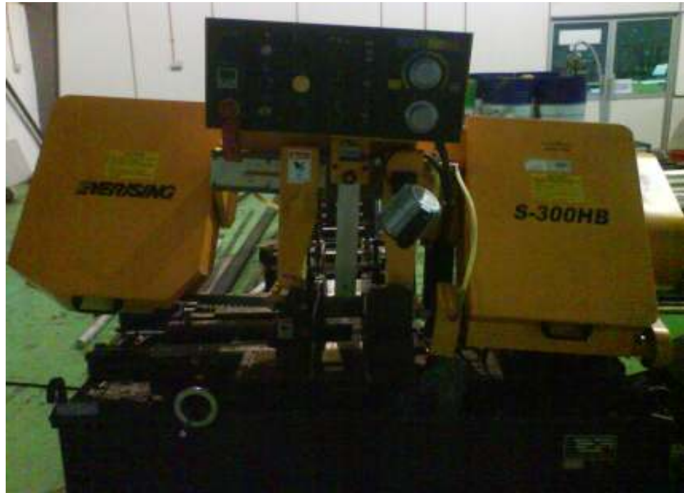
Figure 3.3: Horizontal band saw machine
