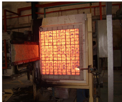
Figure 2: Surface spread of flame test is in progress
