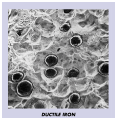
Figure 1.2: microstructure of ductile iron (spheroidal shape)
