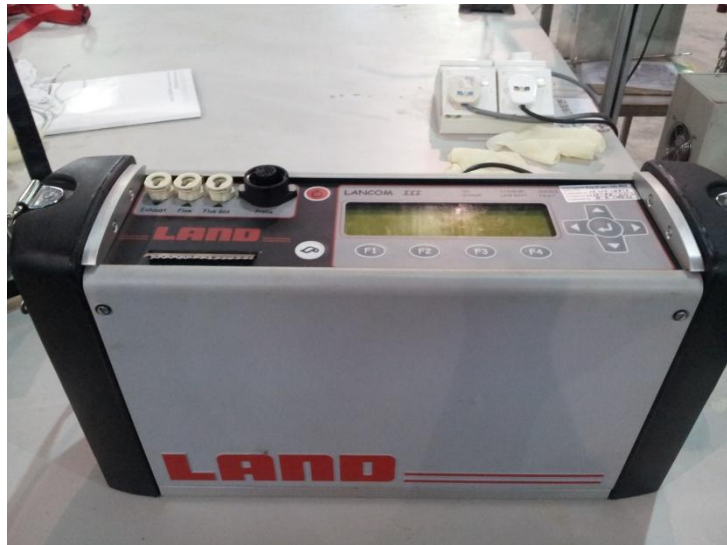
Figure 3-11 : Portable Gas Analyzer.
