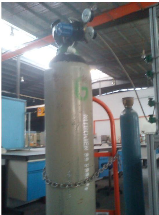
Figure 3-9 : Nitrogen gas cylinder.
