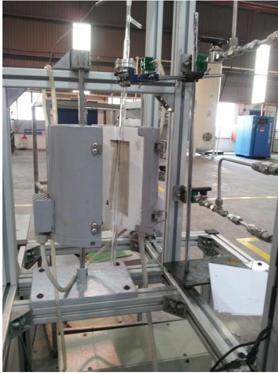
Figure 3-5 : Quartz reactor in tubular furnace.
