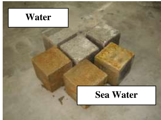
Figure 4 : 1 year water cured OPC cubes with sea water cured specimens
