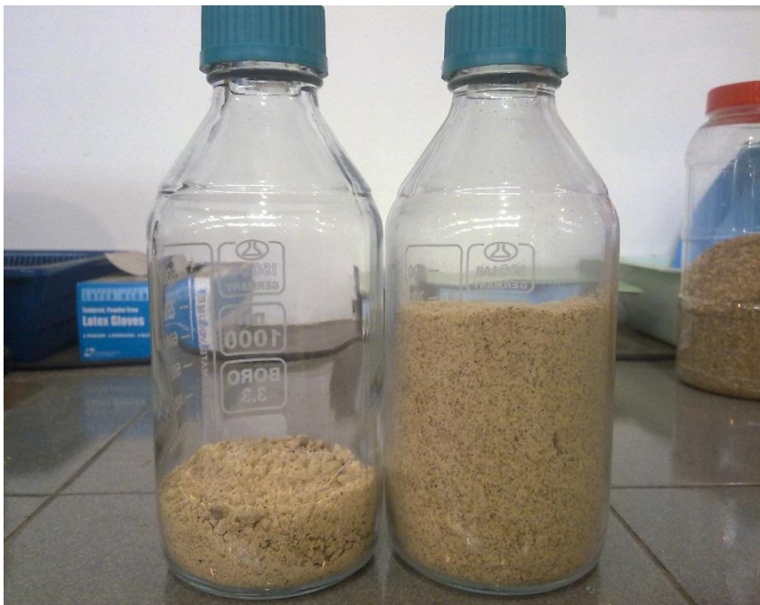
Appendix A.2.1: Moringa oleifera seeds after grinding and sieving
