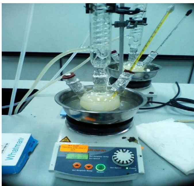
Appendix A.2.6: Mixing of Moringa oleifera oil and methoxide
