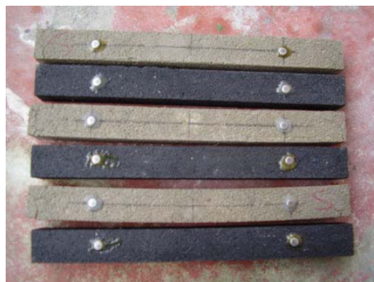
Figure 5. OPC specimen expand more than POFA specimen.
