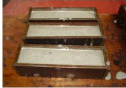
Figure 4 : Slurry Mix In The Mould
