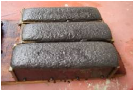
Figure 5 : Slurry Mix After Expansion
