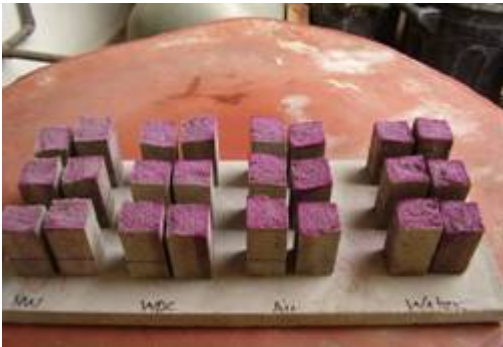
Figure 11 : OPC Aerated Concrete Soon After Phenolphthalein Sprayed
