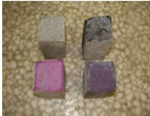
Figure 13 : OPC and POFA Cement Based Aerated Concrete Before And After 24 Hours Of Carbonation Test
