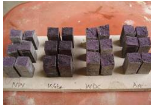
Figure 12 : POFA Cement Based Aerated Concrete 24hrs After Phenolphthalein Reacted
