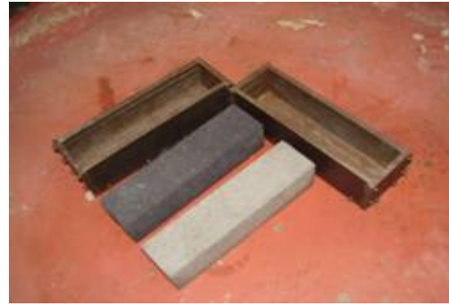
Figure 6 : Specimens After Demoulded
