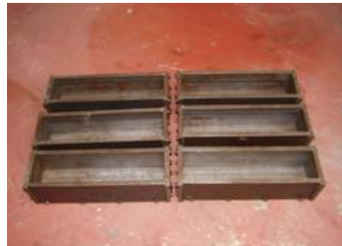
Figure 2: Prisms (40 x 40 x 160mm)
