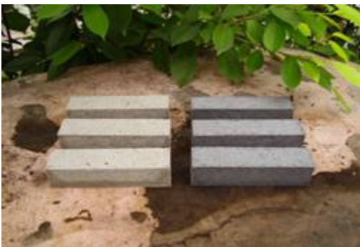
Figure 7 : Natural Weather Curing
