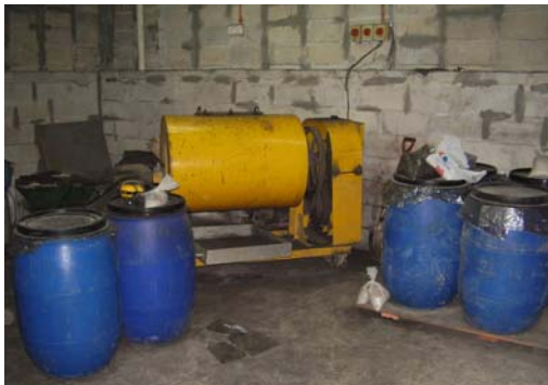
Figure 1: Los Angeles Abrasion Machine For Grinding Ash To Finer Particles
