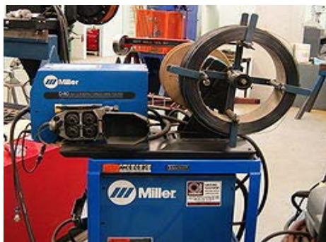
Figure 2.1: Metal Inert Gas (MIG) Welding
