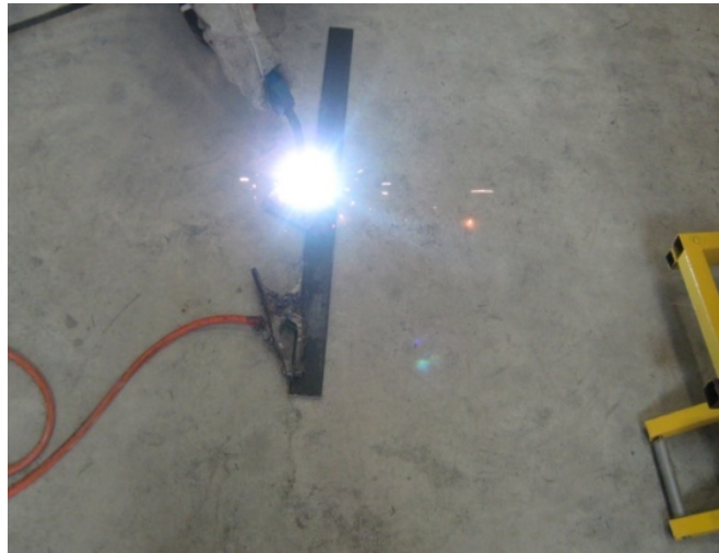
Figure 4.5: Welding process using MIG welding
