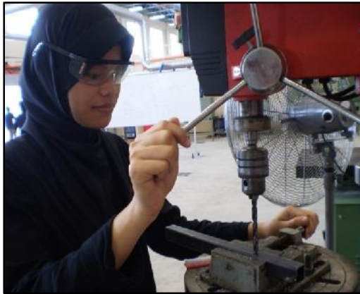
Figure 4.4 Drilling process by using press drill machine
