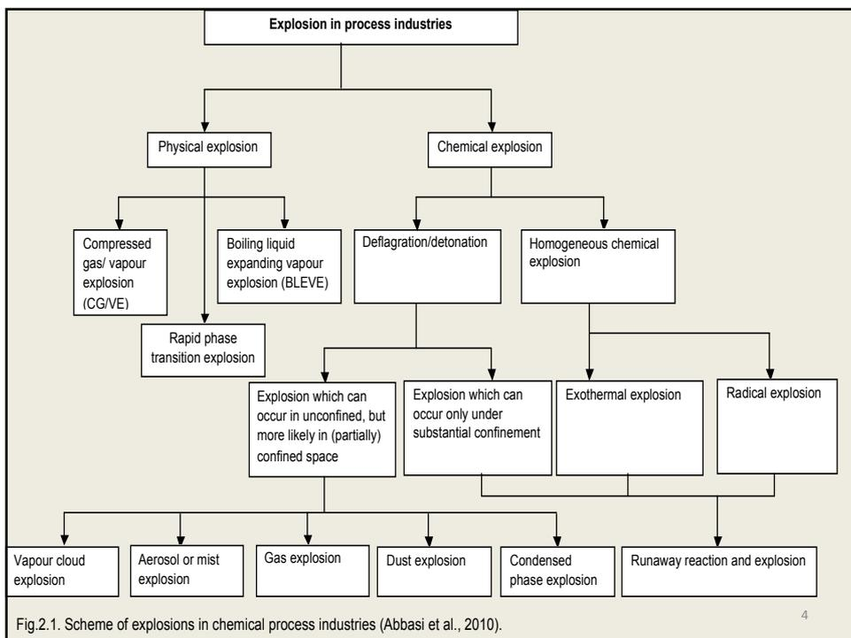
Fig.2.1. Scheme of explosions in chemical process industries (Abbasi et al., 2010).
