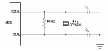
Figure 2.5: Connection of the Crystal to the MCU
