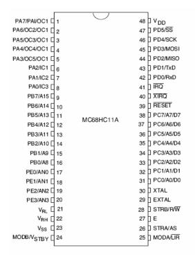
Figure 2.4: Pin Assignment for 48-pin SDIP
