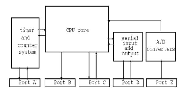
Figure 2.2: Simplified System Block Diagram of 68HC11
